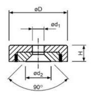
They are assembled with a NdFeB ring magnet and soft steel cover. The Neo magnet can be Nickel or Zinc plated and the steel cover can be Nickel (Zinc or Chrome) plated.
