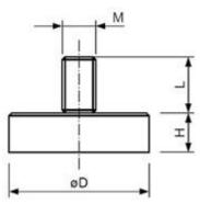
They are assembled with a NdFeB disk magnet and soft steel cover w/bolt on the top. The two parts are bonded together with epoxy. The NdFeB magnet can be Nickel or Zinc plated and the steel cover can be Nickel (Zinc or Chrome) plated.
