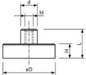
They are assembled with a NdFeB disk magnet and soft steel cover w/tap bolt on the top. The two parts are bonded together with epoxy. The NdFeB magnet can be Nickel or Zinc plated and the steel cover can be Nickel (Zinc or Chrome) plated.
