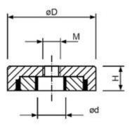
They are assembled with a NdFeB ring magnet and soft steel cover. The Neo magnet can be Nickel or Zinc plated and the steel cover can be Nickel (Zinc or Chrome) plated
