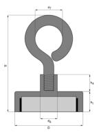
They are assembled with a NdFeB disk magnet and steel eye bolt on the top. The NdFeB magnet can be Nickel or Zinc plated and the steel cover and eye bolt can be Nickel (Zinc or Chrome) plated.
