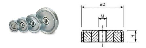
They are assembled with a NdFeB magnet and soft steel cover with internal thread. The NdFeB magnet can be Nickel or Zinc plated and the steel cover can be Nickel (Zinc or Chrome) plated, and the gap filled with a plastic ring
